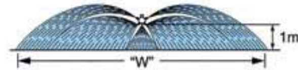
W = Maximum effective coverage with nozzle mounted at 1m height
