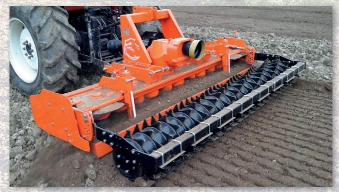
Options include rear cage or packer rollers (packer rollers shown in photo above) and a quick fit blade system.
