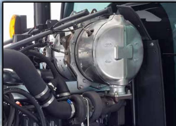
**Diesel Particulate Filter (DPF) Muffler**
