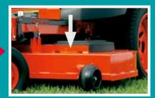
**B** Push and release the pedal again to lower the deck
