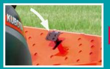
Push and release the pedal to raise the deck
